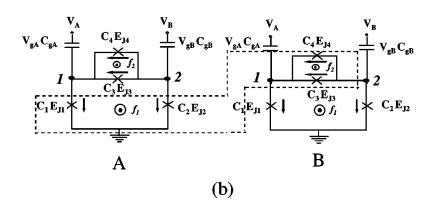
FIG. 7. Coupling of qubits A and B through the mutual inductance between (a) the lower regions of both, and (b) the lower region of A and the upper region of B.
