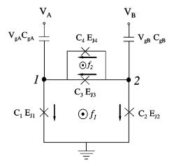
FIG. 6. The four-junction qubit. Two junctions form a SQUID loop and have Josephson energies and capacitance  $\beta$  times larger than the other junctions 1 and 2, which both have Josephson energies  $E_J$  and capacitance C. The nodes A and B represent the superconducting islands that are coupled by gate capacitors  $C_g = \gamma C$  to gate voltages  $V_A$  and  $V_B$ . The arrows define the direction of the currents. The flux is out of the page.
