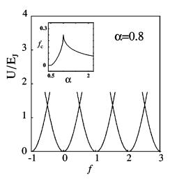
FIG. 2.  $U/E_J$  vs f for  $\alpha = 0.8$  and for minimum energy phase configuration. The energy is periodic with period f = 1 and is symmetric about f = 1/2. Near f = 1/2, there is a region  $[1/2 - f_c, 1/2 + f_c]$  where there are two stable solutions. The inset plots  $f_c$  as a function of  $\alpha$ .
