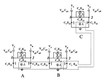
FIG. 8. A method for coupling a single qubit to other qubits.
