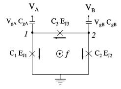
FIG. 1. The three-junction qubit. Josephson junctions 1 and 2 both have Josephson energies  $E_J$  and capacitance C and Josephson junction 3 has a Josephson energy and capacitance  $\alpha$  times larger. The nodes 1 and 2 represent the superconducting islands (nodes) that are coupled by gate capacitors  $C_g = \gamma C$  to gate voltages  $V_A$  and  $V_B$ . The arrows define the direction of the currents. The flux is taken out of the page.
